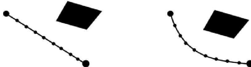
Figure 2-8. Deformable roadmaps. Connections are pushed away by moving obstacles.
