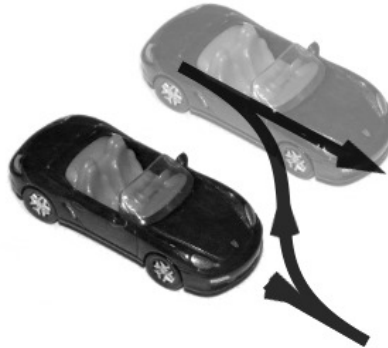
Figure 1-3. An example of non-holonomic constraint. A car cannot go sideways but parallel parking is possible.
