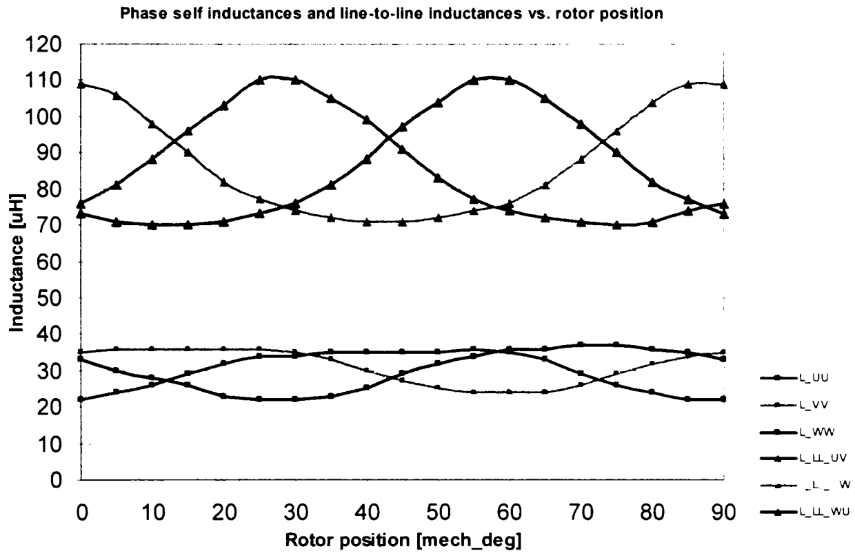
Fig. 5-21 Phase self inductances and line-to-line inductances measured with RLC-bridge (50Hz, 40 mA peak)
