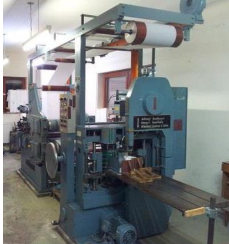
Figure 1.2 40 years old flexographic printing machine for napkin production
