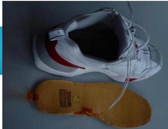
Figure 2.23 Pressure measurement with PVDF sensor in a shoe sole
