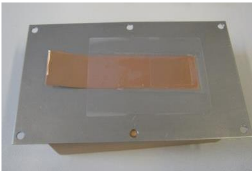
Figure 4.10 Mask on copper film and support steel plate
