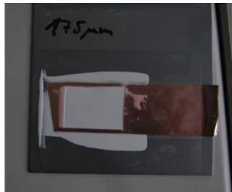
Figure 4.11 Sensor after applying PZT-paint
