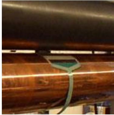
Figure 2.2 Measuring nip roller with Tekscan sensors
