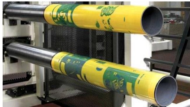
Figure 1.10 Sleeve with printing plate
