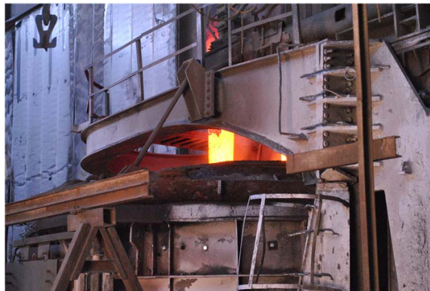
Fig.2.8. Cuptor electric cu arc, capacitate 50 tone.
