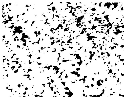
Fig. 3.3. Oțel RCA 37 (Nital 3%, 100:1)
