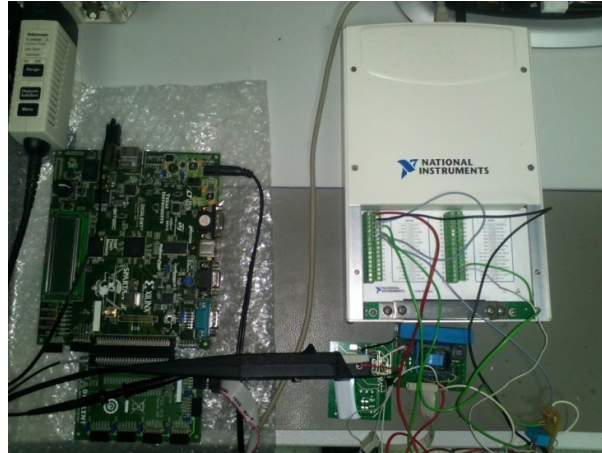
Figure 5.46 Experimental setup: Cuk converter, SPARTAN FPGA, NI DAQ board. Source [original]
