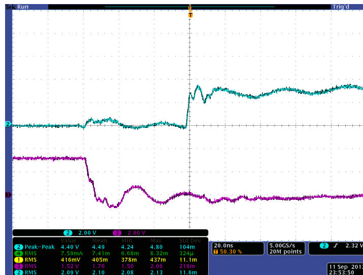
Figure 5.45 Oscilloscope view of the FPGA control signals output with 5 ticks delay (62.5ns). Source [experiment]
