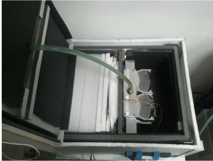
Figure G.3 TEM test rig placed in the thermally isolated chamber. Source [original]
