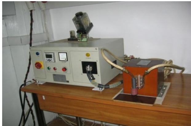
Figure 4.6: The heating/melting 12 Kw equipment
