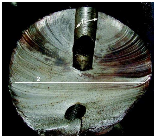
Figure 1.19: A basic fatigue failure complicated by several holes (adapted from [54])
