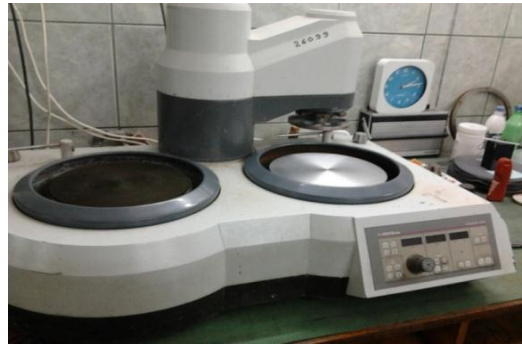
Figure 4.8: Phoenix 4000 polishing machine
