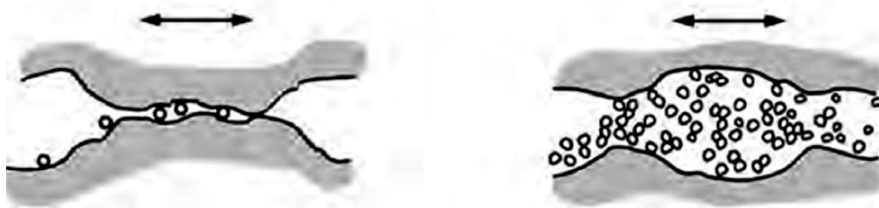
Figure 1.14: Chemical wear process (adapted from [1])
