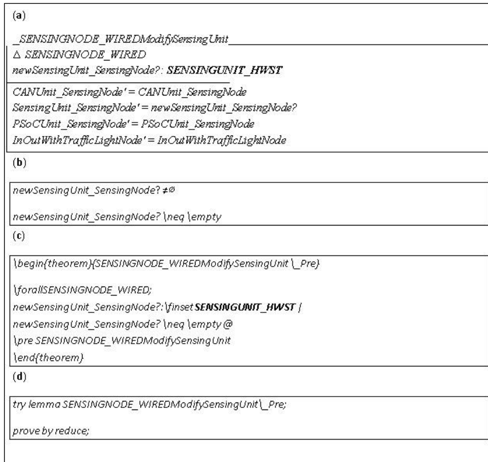
Figure 26 (a) Z specification of ModifySensingUnit operation; (b) Z language statements for sensing node model; (c) Z language statements for sensing node model; (d) Z language evaluation of sensing node theorem
