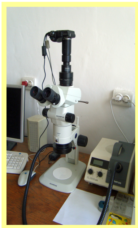
Fig. 3.63 Stereomicroscopul OLYMPUS SYX7.
