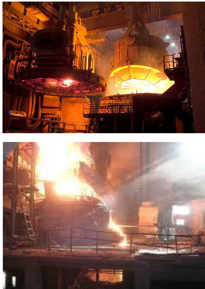
Fig.2.5.Cuptor electric cu arc, capacitate 50 ton
