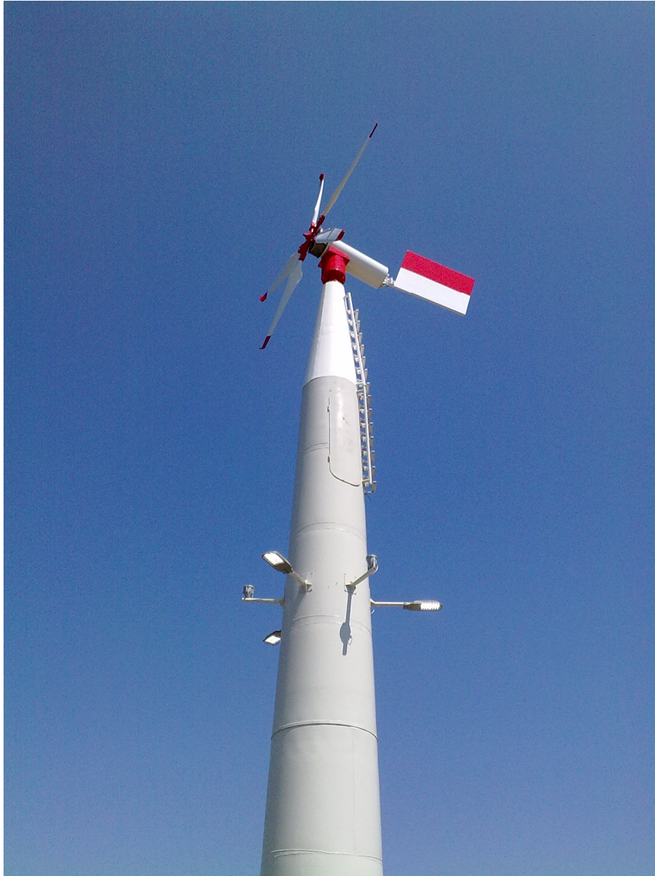
Fig.2.9. The five blades variable-speed wind turbine.
