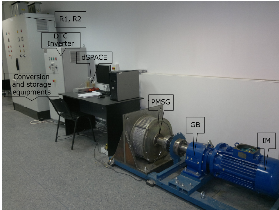
Fig.6.1. The complete laboratory setup.
