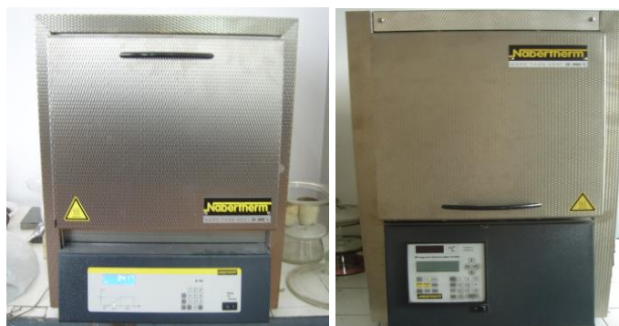
Fig. 4.13. Cuptoare de topire –a) cuptor de topire (calcinare) Nabertherm model L15/12/B180; b) cuptor de topire (calcinare) Nabertherm model LHT 02/17
