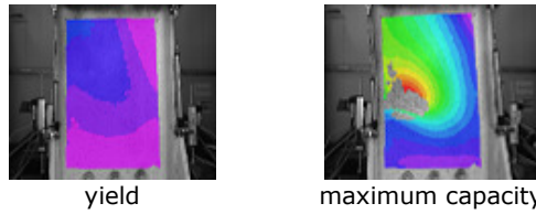
Fig. 5-58. Out of plane deformation of beam web (Vic 3D)
