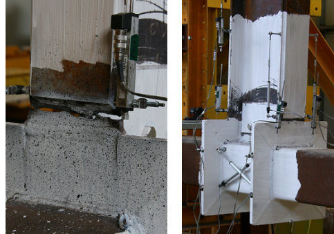
Fig. 5-72. S700-RBS-R-M joint: monotonic response and illustration of the failure mode
