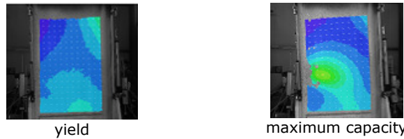
Fig. 5-63. Out of plane deformation of beam web (Vic 3D)
