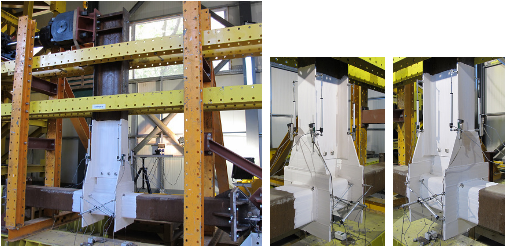
Fig. 5-61. S700-CP test assembly and connection zone – before test
