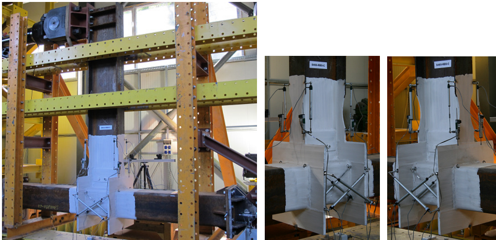
Fig. 5-46. S460-RBS test assembly and connection zone – before test
