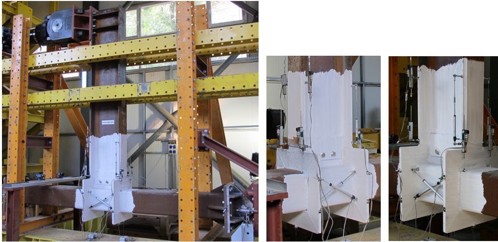
Fig. 5-71. S700-RBS-R test assembly and connection zone – before test
