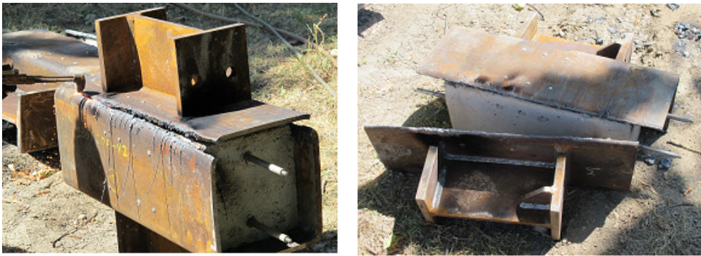
Fig. 5-31. Flame cutting of the concrete filled tubes
