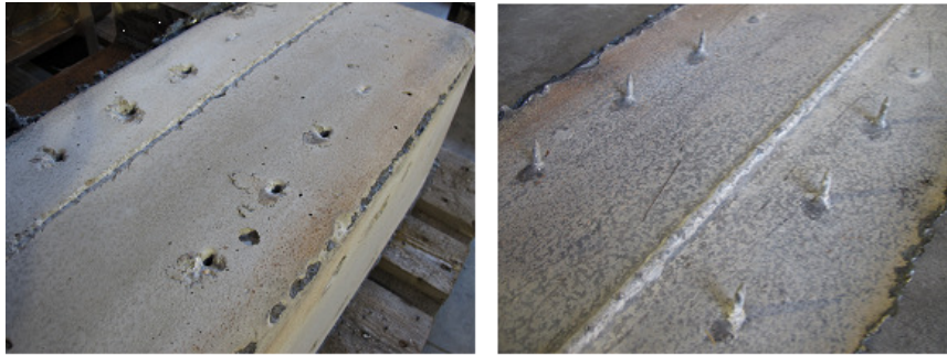
Fig. 5-33. Response of concrete and connectors to monotonic loading
