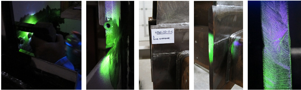
Fig. 5-107. Magnetic particle testing (S460-RBS-R-C, and S700-CP-R-C)
