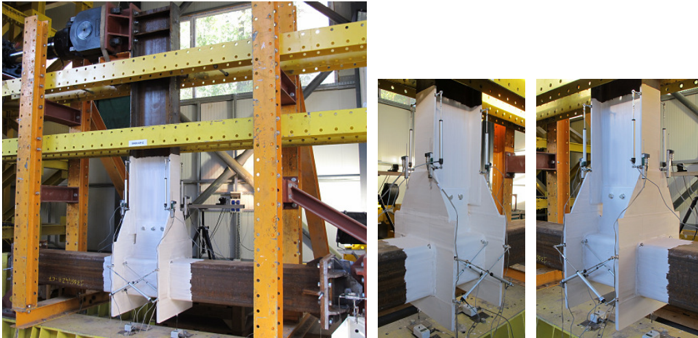
Fig. 5-56. S460-CP test assembly and connection zone – before test
