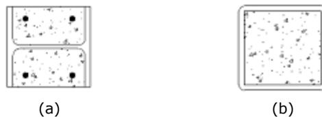
Fig. 3-6. Composite column: (a) partially encased wide flange section, and (b) concrete filled rectangular hollow section [1]
