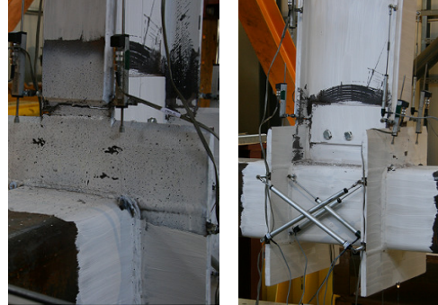
Fig. 5-67. S460-RBS-R-M joint: monotonic response and illustration of the failure mode
