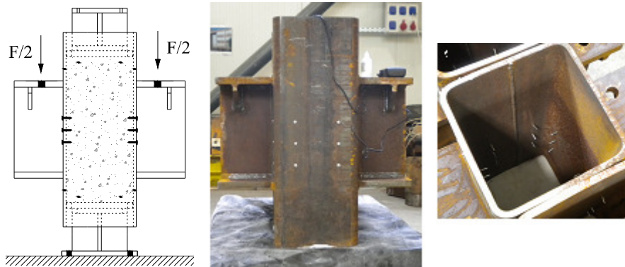
Fig. 5-2. Specimen configuration for the load introduction tests
