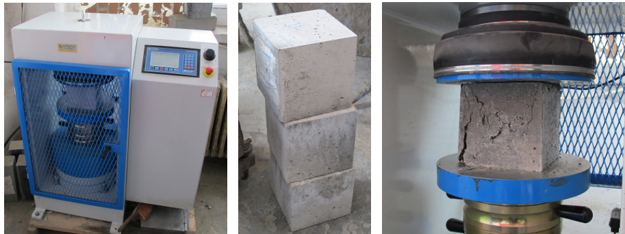
Fig. 5-14. Testing device and concrete cubes (before and after compression test)
