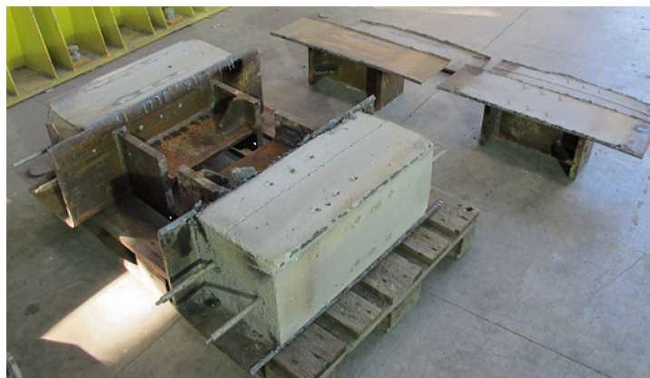
Fig. 5-32. Specimens (S460-F-H-C / S460-F-H-M) with removed tube faces
