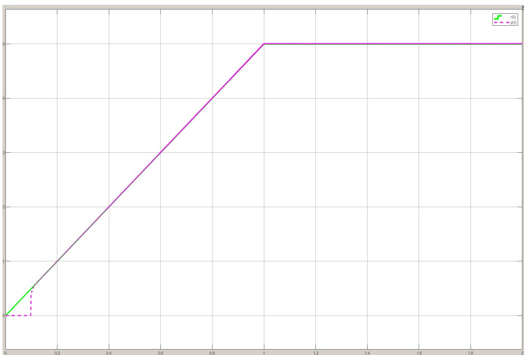
Figure 2.26: Simulation results of input-output signal with current ramp slope 5A/S and from 0s-2s [original]
