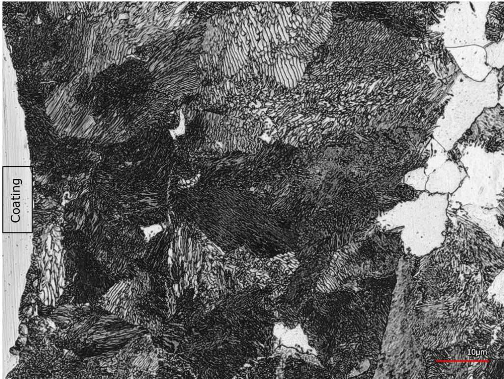
Figure 4.28 Sorbite lamellar structure on the interface with perlite-ferite inclusions
