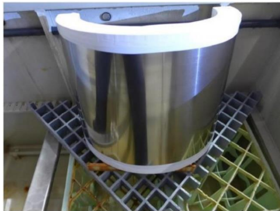
Figure 4.53 Sample before salt spray test
