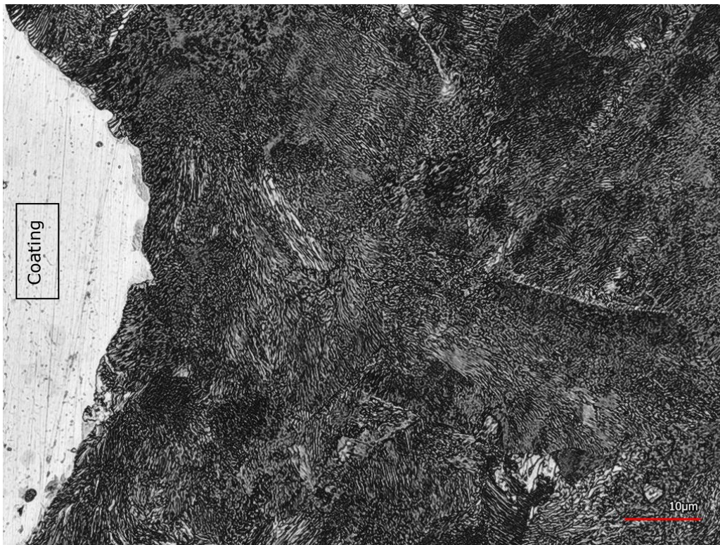
Figure 4.30 Sorbite lamellar structure on the interface
