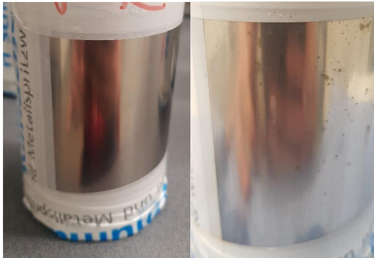
Figure 4.58 KS-IC-45 before(left) and after (right) salt spray test
