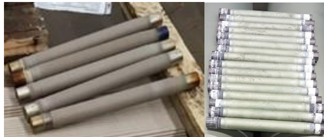
Figure 4.8 As-sprayed (left) and remelted (right) bars
