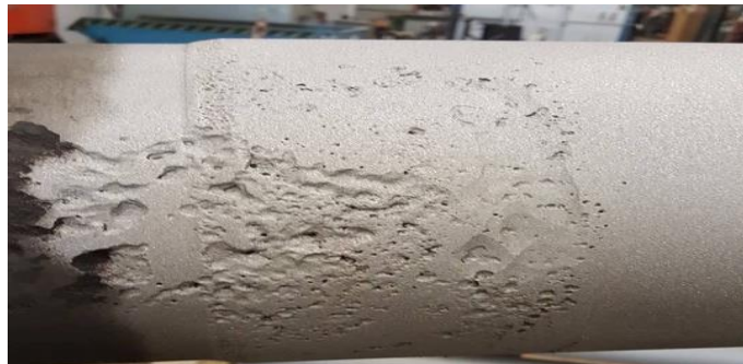
Figure 4.50 Corroded cylinder sample
