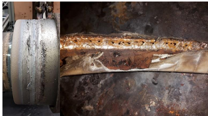
Figure 4.24 Element and coating destruction
