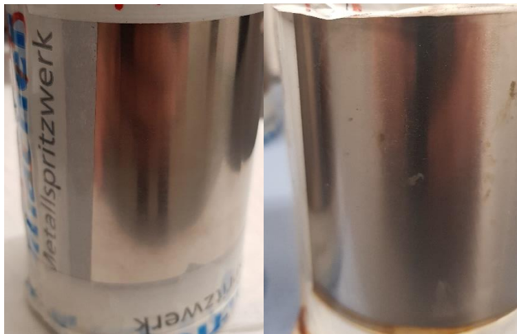
Figure 4.60 KS-IC-55S before(left) and after (right) salt spray test
