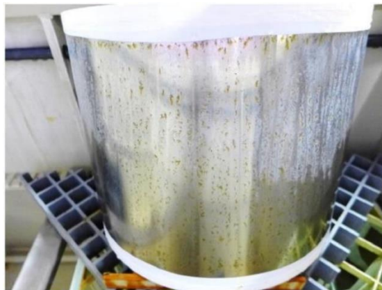
Figure 4.55 KS-IC-45 after 480 hours Salt spray test
