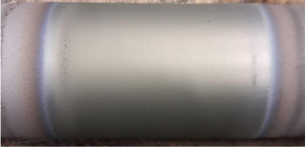
Figure 4.19 Sample remelted with rectangular cross element section
