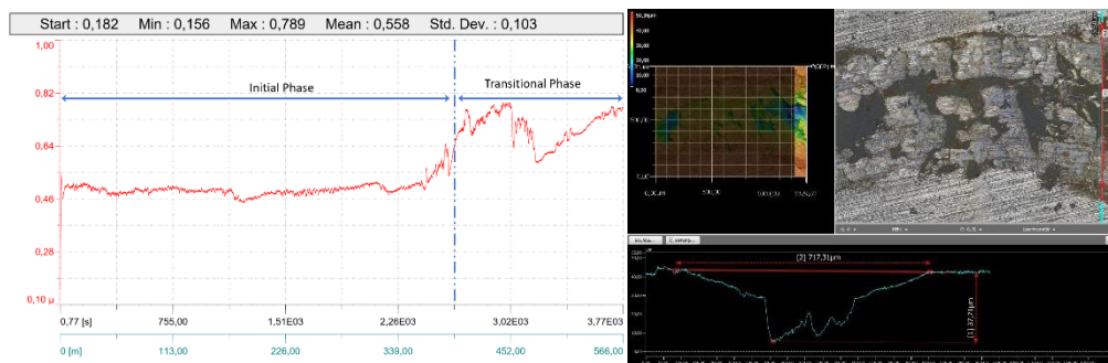
Figure 4.13 Friction coefficient and wear track of as-sprayed KS-IC-55
