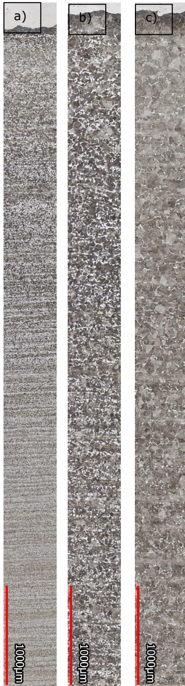
Figure 4.25 Substrate structure a) 7mm b) 12mm c) 20mm working distance
