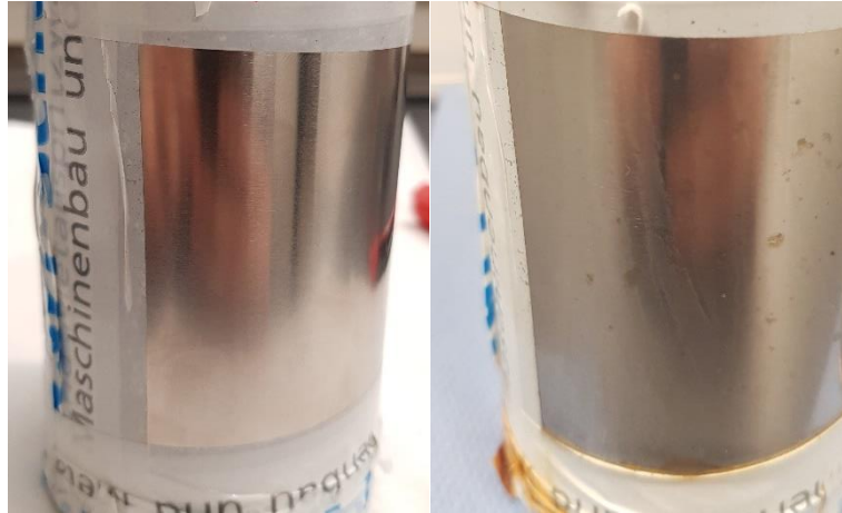
Figure 4.61 KS-IC-55 before(left) and after (right) salt spray test
