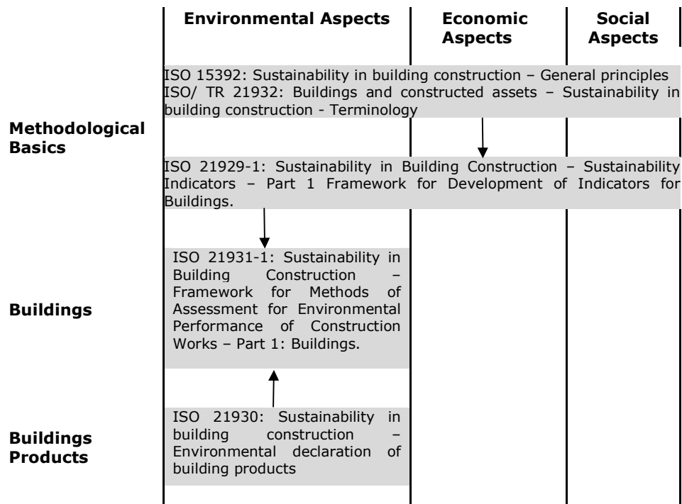
Figure 2.3. Suite of related International Standards for sustainability of buildings and construction works [18]
