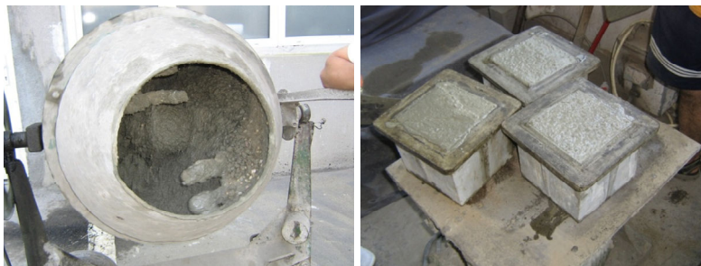
Figure 6.3. Preparation of the concrete mixtures
