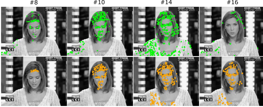
Figure 5-5. Tracking of sparse OF features on the TV show sequence. 1 st row - sparse OF features, 2 nd row - set \mathcal{D} of tracked features
