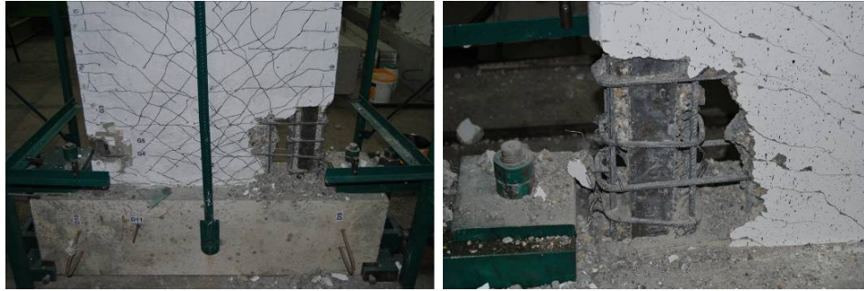
a) General view b) Compression zone Figure 4.15 Details of specimen CSRCW2 at the end of the test
