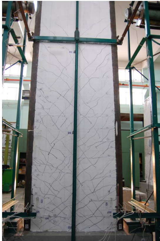
Figure B.33 Specimen CSRCW5 at 40 mm drift
