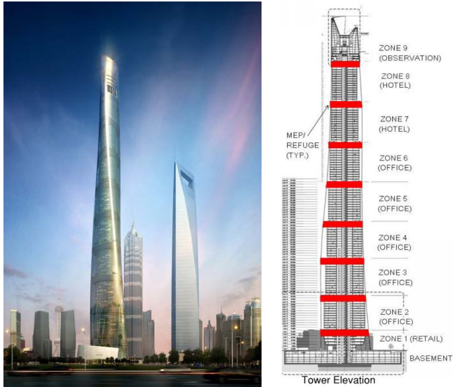
Figure 2.34 Shanghai Tower rendered view and elevation
