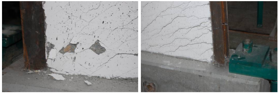
a) Compression zone b) Tension zone Figure 4.21 Details of specimen CSRCW5 at failure
