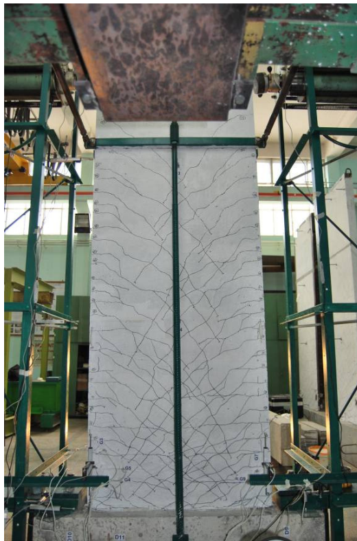
Figure B.9 Specimen CSRCW2 at 40 mm drift
