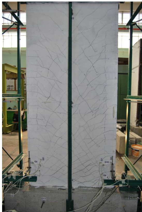
Figure B.25 Specimen CSRCW4 at 40 mm drift
