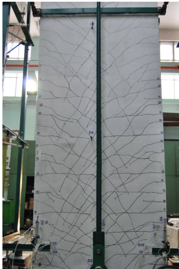
Figure B.17 Specimen CSRCW3 at 40 mm drift
