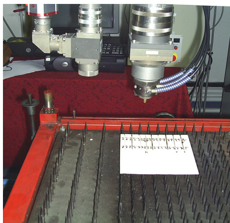
Fig 2.8 Laser cu Nd :YAG de Tip TRUMPH HL124P, P_{\max} = 150W
