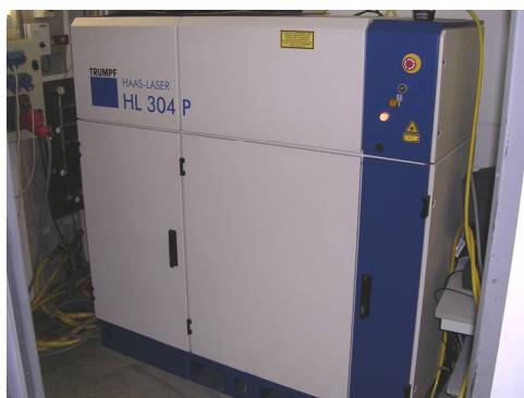
Fig. 2.9 Laser cu Nd :YAG de tip TRUMPH HL304P, P_{\max} = 400W
