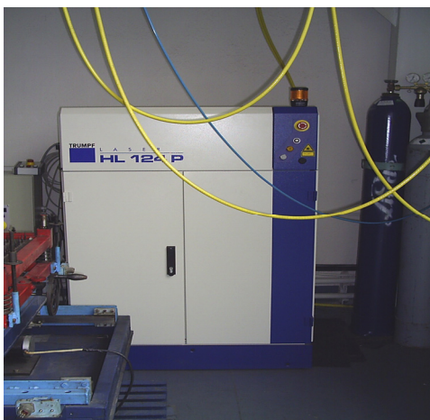
Fig 2.8 Laser cu Nd :YAG de Tip TRUMPH HL124P, P_{\max} = 150W
