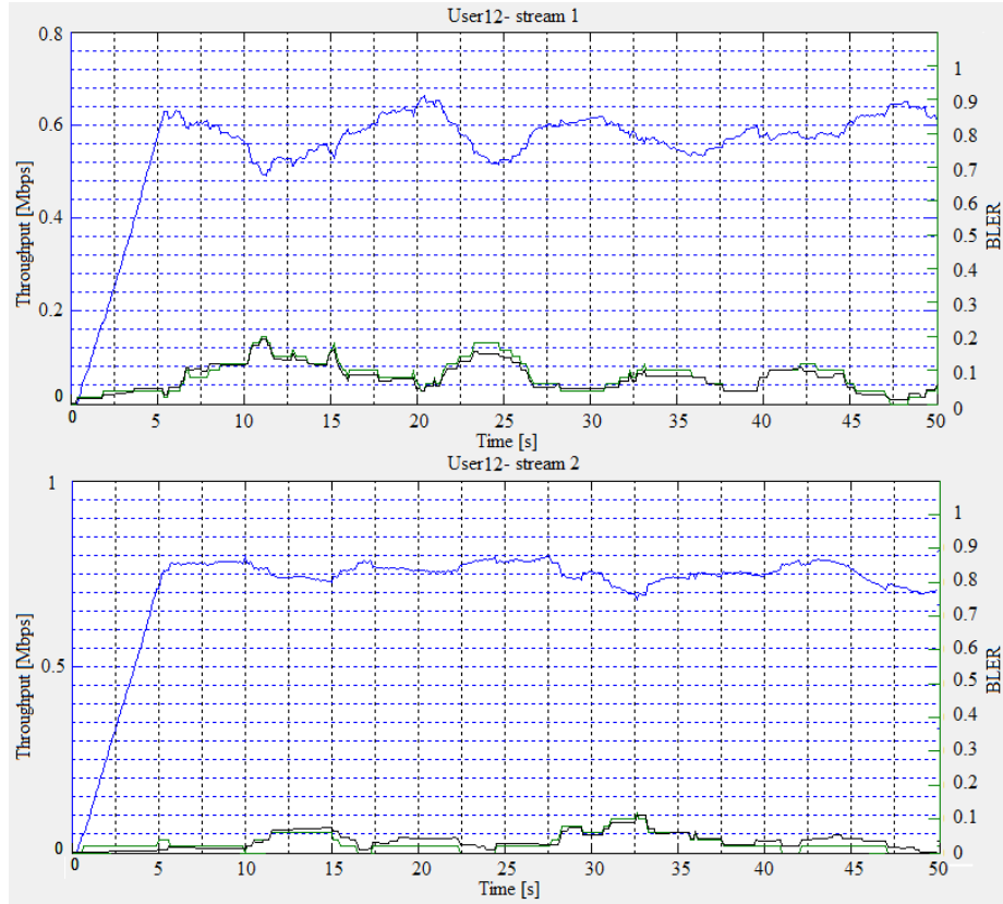
Figure 61 - Throughput and BLER for User 12 when RR scheduler and LTE delivery mechanism are used
