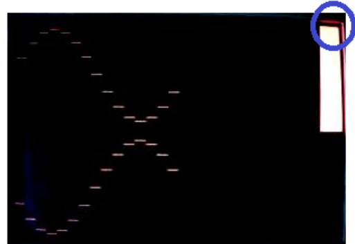
Fig. 4.9 The transmitted signal if the input is 0
