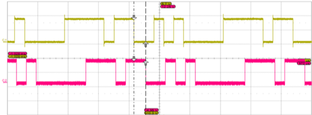
Fig. 5.23 The waveforms: (a) The modulating signal; (b) The demodulated signal
