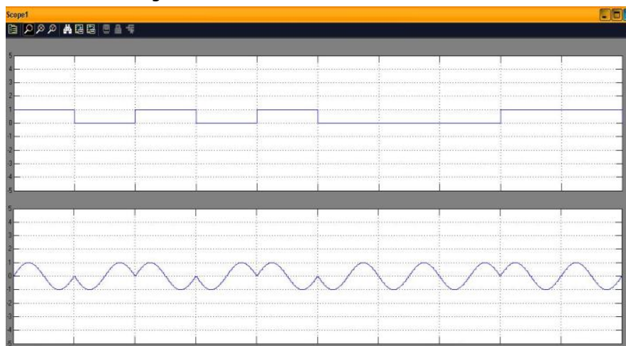
Fig. 4.16 The modulating and modulated signals
