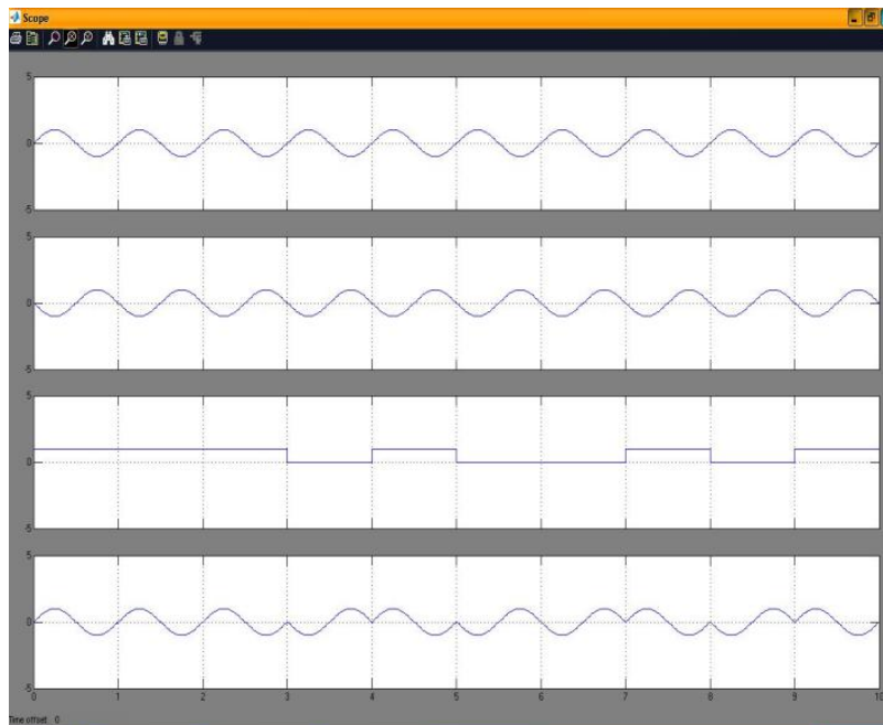
Fig.4.13 The waveforms on the scope: (a) Sine; (b) -Sine; (c) Modulating signal; (d) Modulated signal
