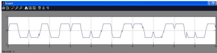
Fig. 4.37 The signal at the output of the saturation block
