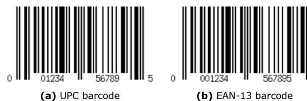
Figure 1.3: UPC barcode invented by IBM and the EAN-13 barcode that is composed of a UPC and a prefixed zero.
