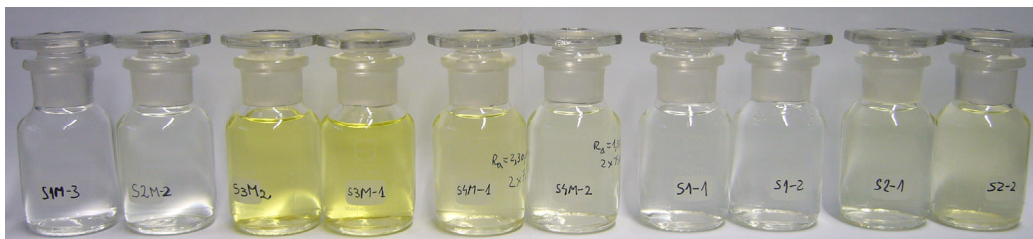
Figure A.5 An visual aspect of the water resulted after electrochemical corrosion tests (WC-Co-Cr coatings: S1M-3 fine*; S2M-2 medium*; S1-1 and S1-2 coarse*) (WC-Cr 3 C 2 -Ni coatings: S3M1 and S3M2 fine*; S4M-1 and S4M-2 medium*; S2-1 and S2-2 coarse*) * the type of powder used for the corresponding coating
