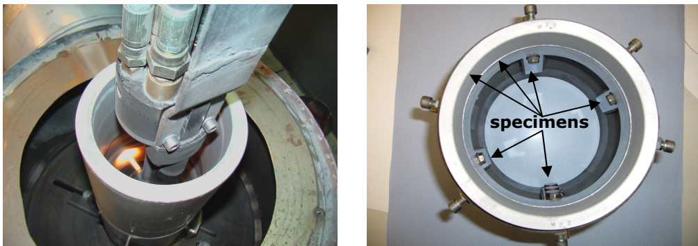
Figure 3.21 Special test set-up for internal coatings using ID CoolFlow Mono Gun; sample holder
