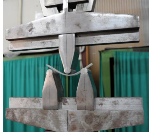
Figure 2.48 Three point bending support with PA-12 specimen
