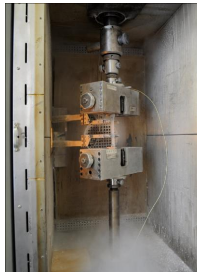
Figure 2.2 Thermal chamber on Zwick Z250 machine
