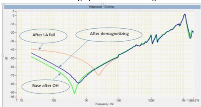
Fig. 8. SFRA of H.V. winding after demagnetization
