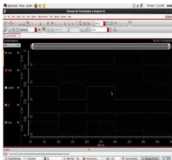
Fig. 2. 2 Simulation output of Full Adder
