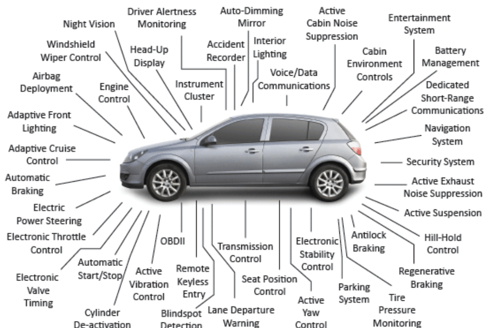
Figure 1.1. Electric and electronic device systems on the modern cars [1.1]
