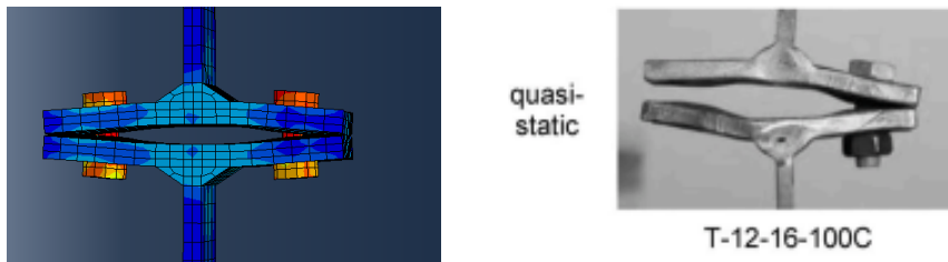
Figure 5. 16. Failure of T-stub specimen in the numerical model M1_20_Q, at normal temperature, under quasi-static strain rate.
