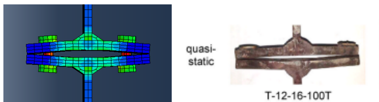
Figure 5. 20. Failure of T-stub specimen in the numerical model M3_542_Q, at 542 °C, under quasi-static strain rate.
