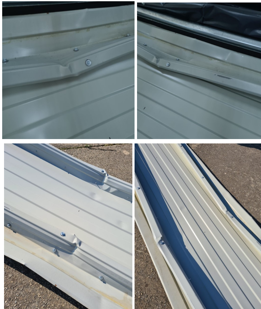
Figure 7.7 LT-RO-P specimen after the experimental test - extension to Figure 7.6
