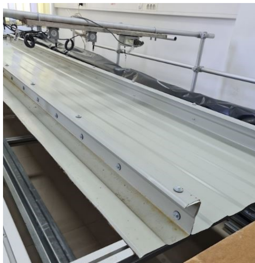
Figure 3.22 Restrained-opened liner trays prepared for wind tests: a) LT-RO-S and b) LT-RO-P
