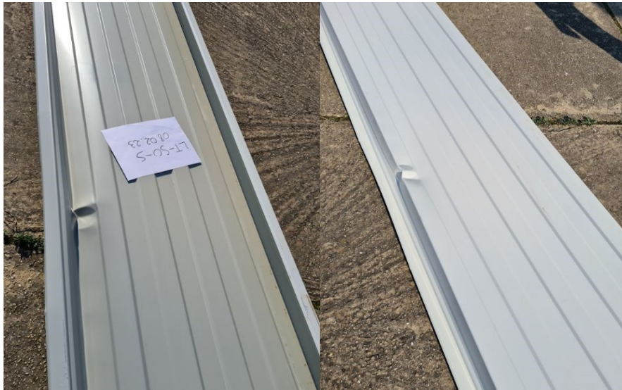
Figure 3.50 LT-SO-S specimen after failure: typical non-symmetric failure at mid-span
