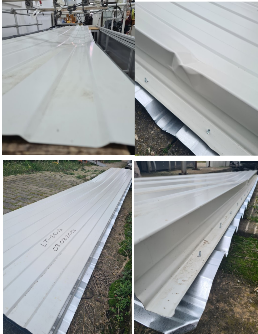
Figure 7.11 LT-SC-S specimen after the experimental test – extension to Figure 7.10
