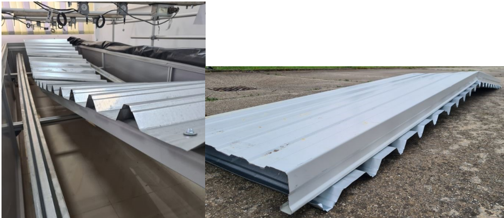
Figure 3.38 LT-SC-P liner tray specimen after failure: showing failure at mid-span
