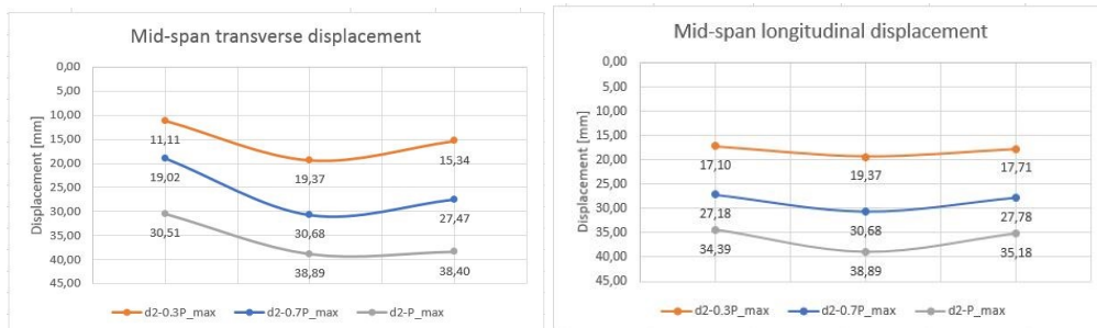
Figure 3.28 Displacements of the LT-SO-P liner tray during the test
