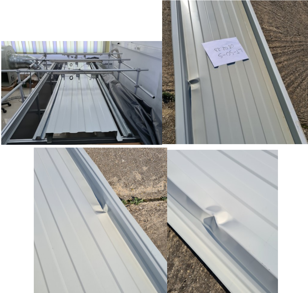
Figure 7.9 LT-SO-S specimen before (up-left) and after (up-right and down) experimental test
