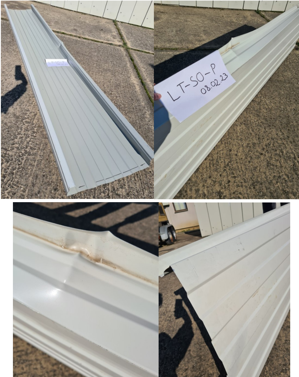
Figure 7.1 LT-SO-P specimen after experimental test
