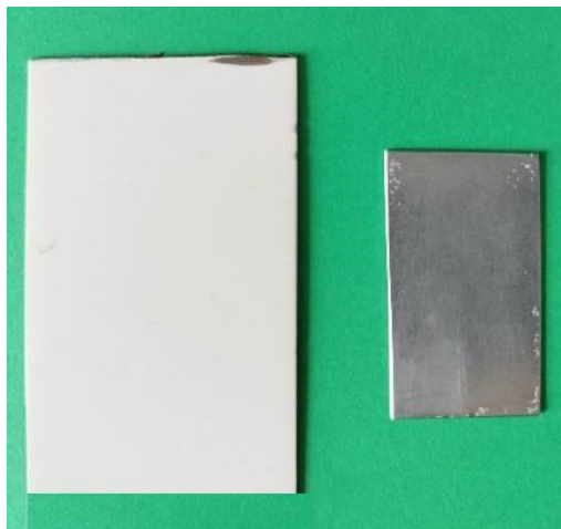
Figure 3.71 Steel sample before (left) and after (right) removing the paint coating
