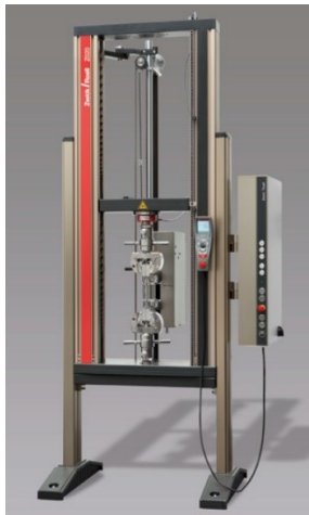
Figure 3.66 Illustration of tensile testing machine
