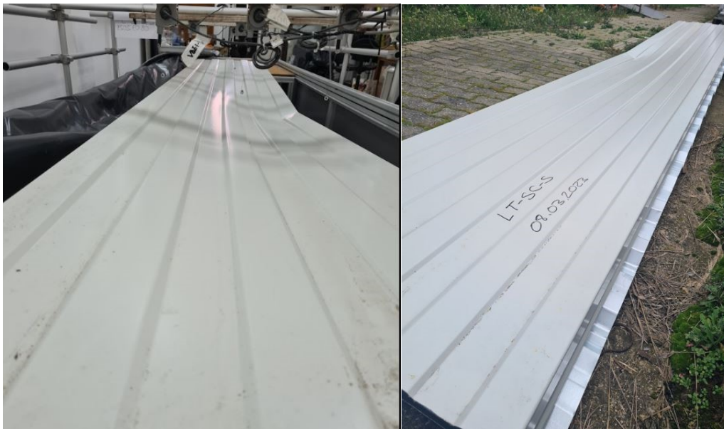
Figure 3.54 LT-SC-S liner tray specimen after failure: typical non-symmetric failure at mid-span
