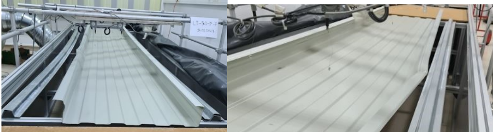
Figure 3.33 LT-SO-P-P liner tray specimen after failure: showing typical non-symmetric failure at mid-span
