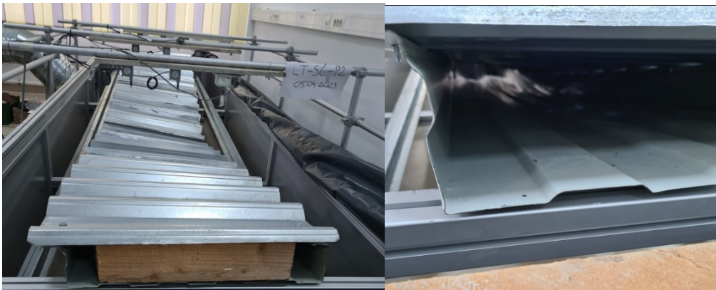
Figure 7.3 LT-SC-P specimen after the experimental test
