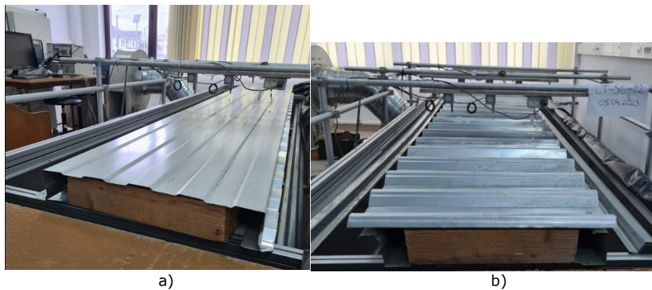
Figure 3.18 Simple-closed liner tray specimens prepared for wind tests: a) LT-SC-S and b) LT-SC-P
