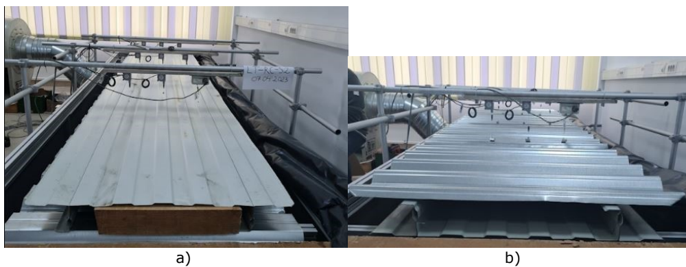
Figure 3.23 Restrained-closed liner tray specimens prepared for wind tests: a) LT-RC-S and b) LT-RC-P
