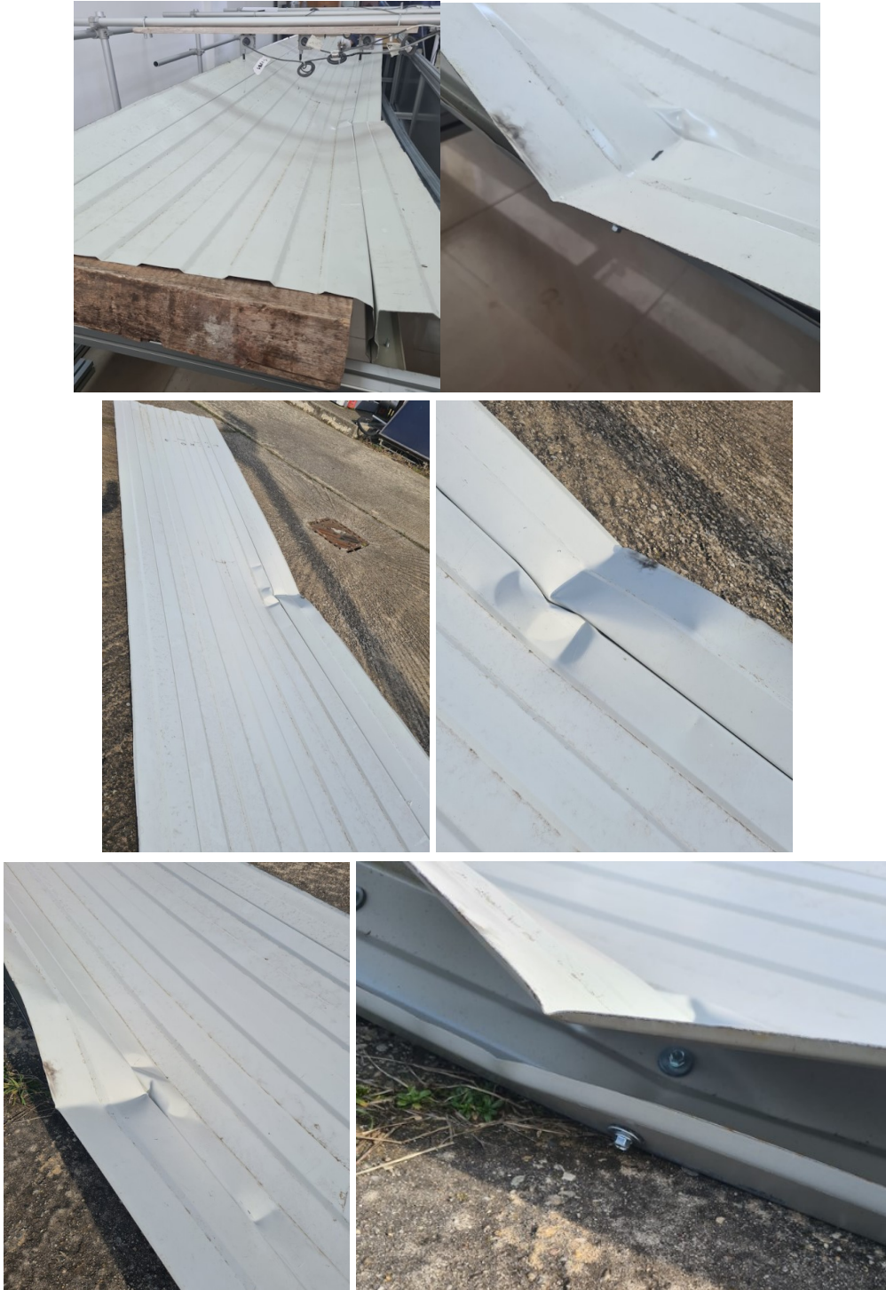
Figure 7.12 LT-RO-S specimen after experimental test
