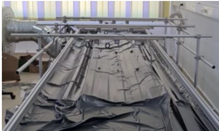
Figure 3.20 Video caption of the strong deformation of the wide flange in the support area, during the first test of liner trays subjected to wind suction
