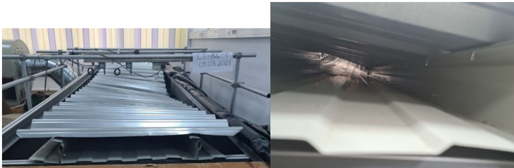
Figure 3.46 LT-RC-P liner tray specimen after failure: showing failure at mid-span
