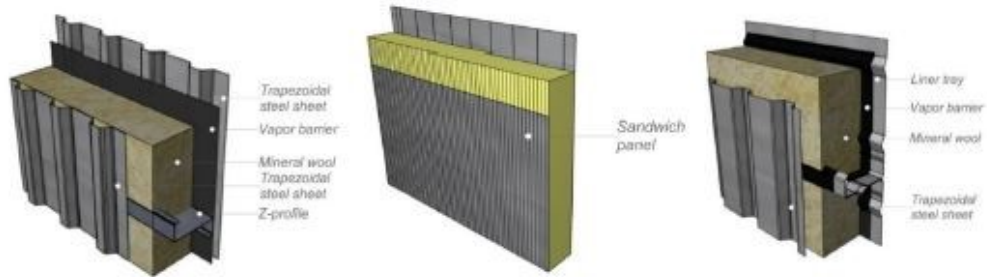
Figure 2.11 Built-up wall system (left), sandwich panel wall system (middle) and liner tray wall system (right) [31]
