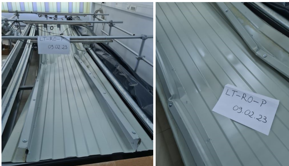
Figure 3.42 LT-RO-P liner tray after failure: showing failure at mid-span
