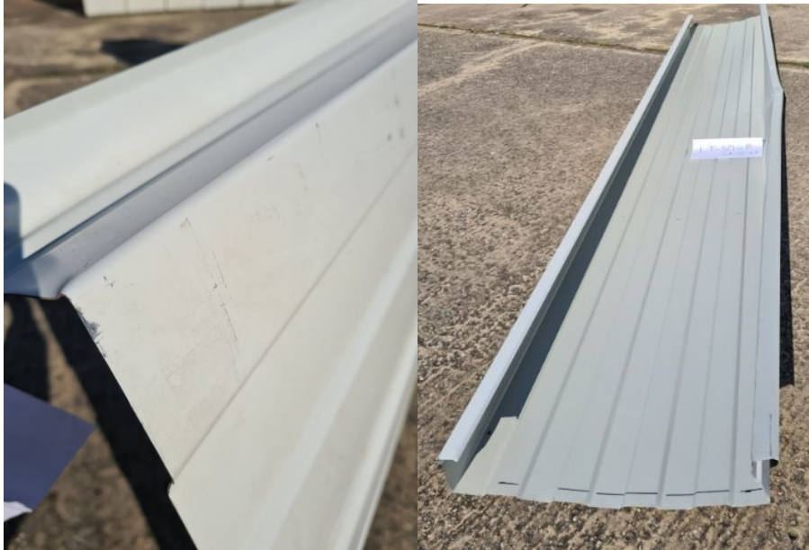
Figure 3.29 LT-SO-P specimen after failure: local buckling of the wide flange in the support area (left); typical non-symmetric failure at mid-span (right)
