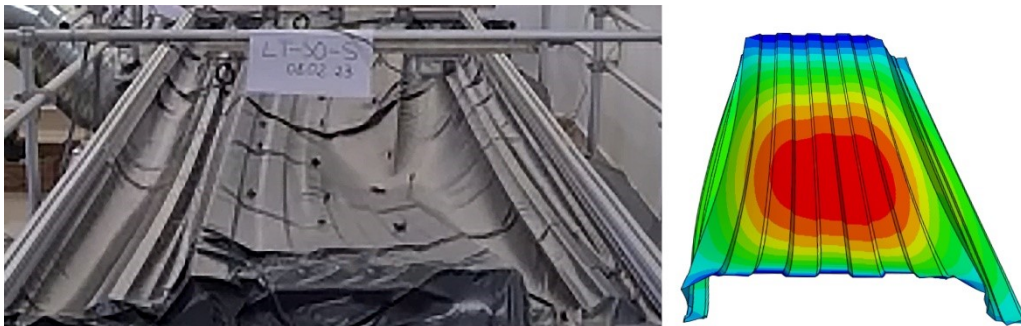
Figure 4.28 LT-SO-S specimen after failure at P_{\max\_exp} = 1044.27 Pa (left) and simple-opened liner tray FEM model subjected to suction at P_{\max\_exp} = 1044.27 Pa (right)
