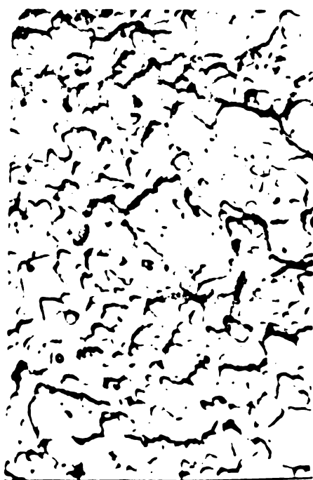
Fig.3. M.E.x 2700 Călire+Rev. 160^{\circ}\text{C}
