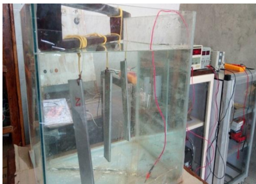
Fig. 2.b. The electrolytic tank with pure water ( \rho = 25 \Omega \cdot m ), steel and zinc segments.
