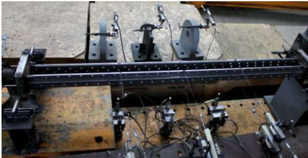
Fig. 3.32 Test setup for interactive buckling specimens
