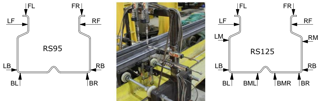
Fig. 3.17 Measuring device for geometric imperfections
