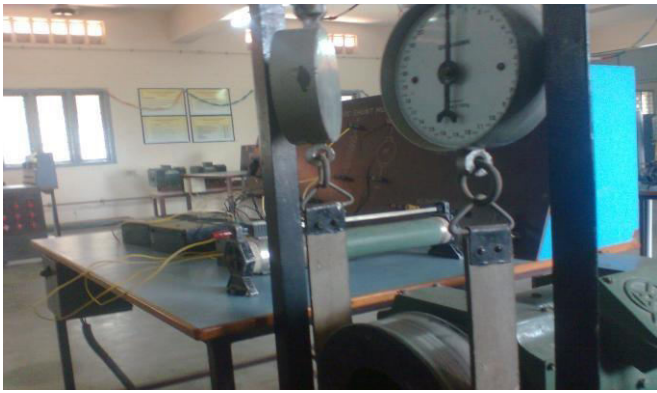
Fig.5. Laboratory experiment set-up model of D.C motor drive system at various speed control methods.
