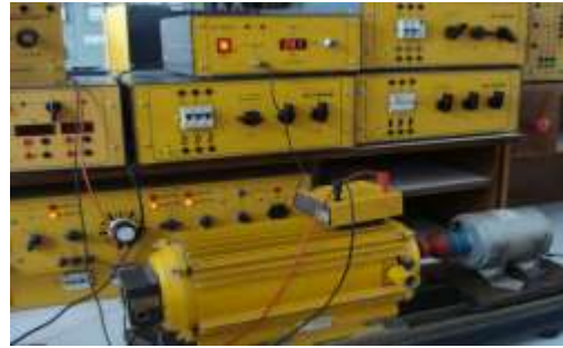
Figure 10 Experimental Setup for acquiring motor characteristics.
