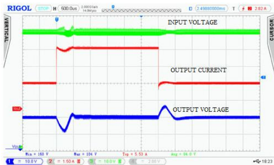
Fig. 18. (b). Transitory response of the resonant converter versus step changes in output load by: (Spectator controller.
