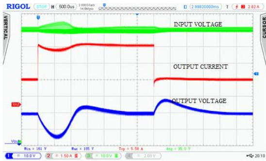
Fig. 18. (a). Transitory response of the resonant converter versus step changes in output load by: (PID controller,)
