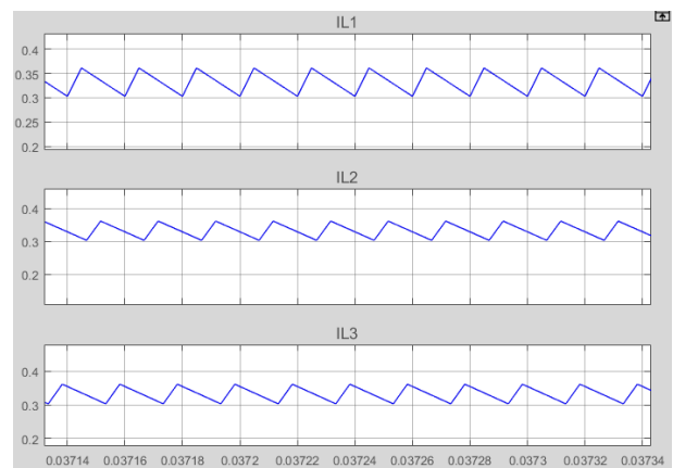
Fig. 19 Inductor currents of 3-phase Boost converter
