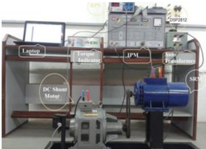
Figure 4. photograph of Experimental test bench
