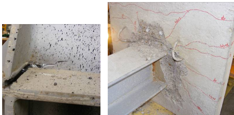
Fig. 3.70. Failure of the DB-Comp1 & 2 specimens
