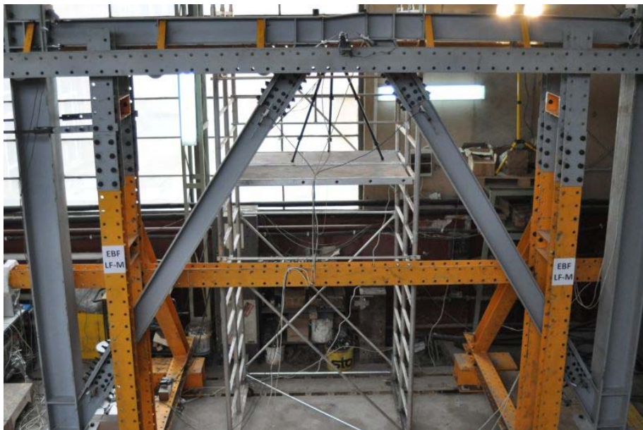
Fig. A.14. EBF at the initiation of yield in link
