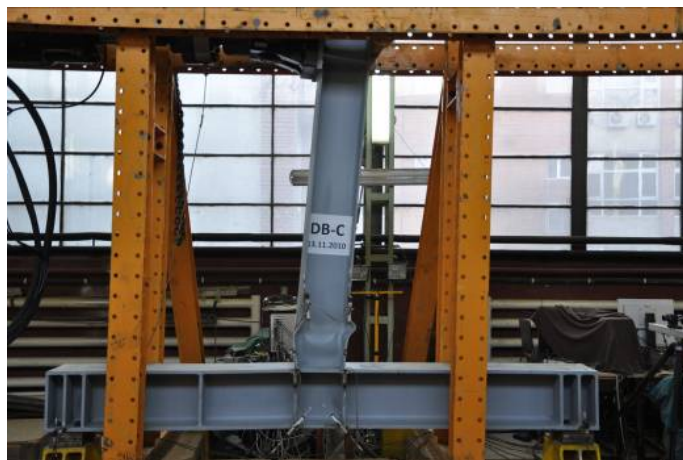
Fig. A.18. Cyclic testing of the joint with RBS
