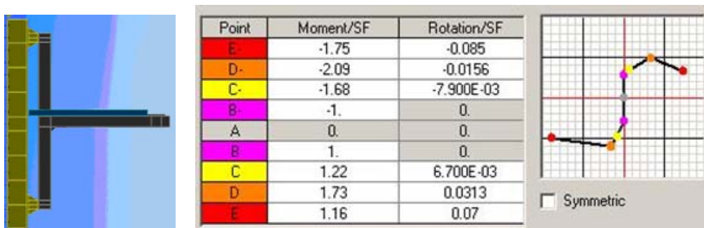
Fig. 4.5. Plastic hinge model proposed for the composite RBS
