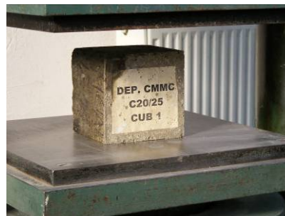
Fig. 3.23. Testing of the concrete cubes
