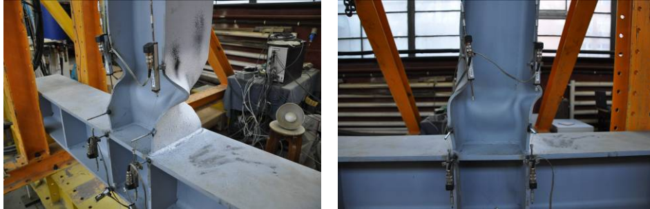
Fig. 3.75. Buckling of the flanges in the RBS for specimen DB-C RLD
