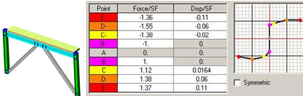
Fig. 4.6. Plastic hinge model proposed for the composite short link
