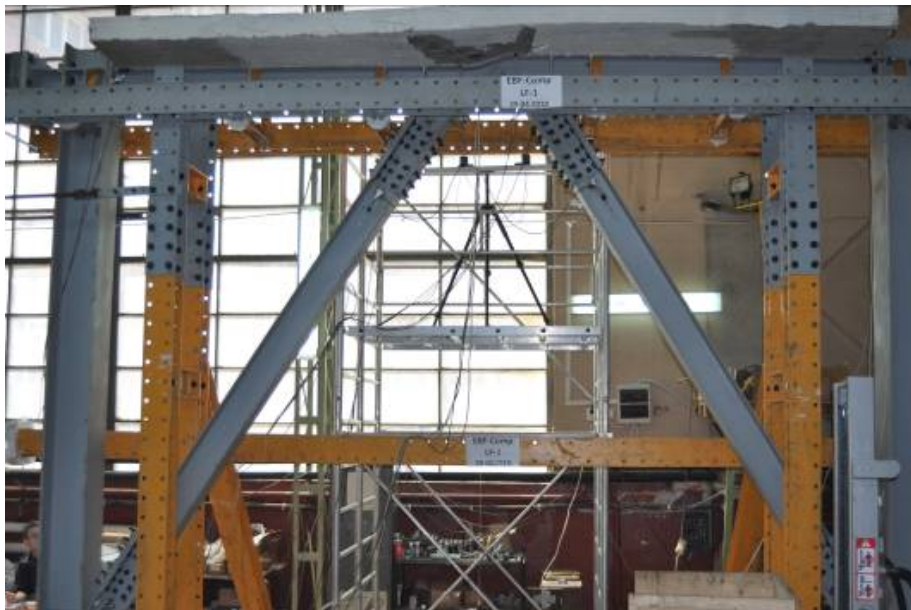
Fig. A.16. Test setup for the EBF with composite beam
