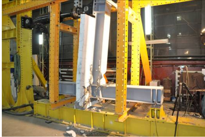
Fig. A.20. Cyclic testing of the composite joint with RBS
