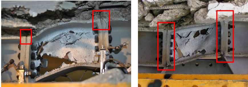
Fig. 3.54. Pinching effect on the link-to-beam connection
