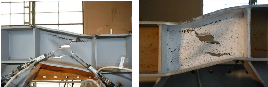
Fig. 3.39. Behaviour of the link, failure of the web in shear
