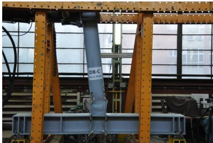
Fig. A.19. Cyclic testing of the joint with RBS
