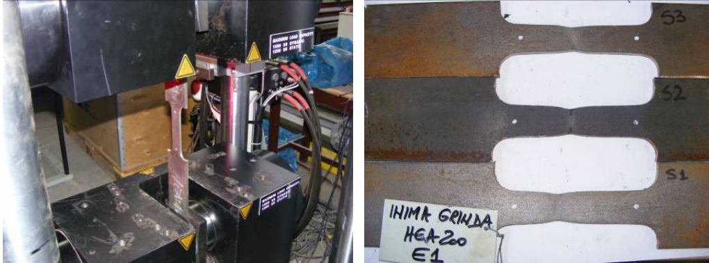
Fig. 3.21. Tension testing of the flat specimens
