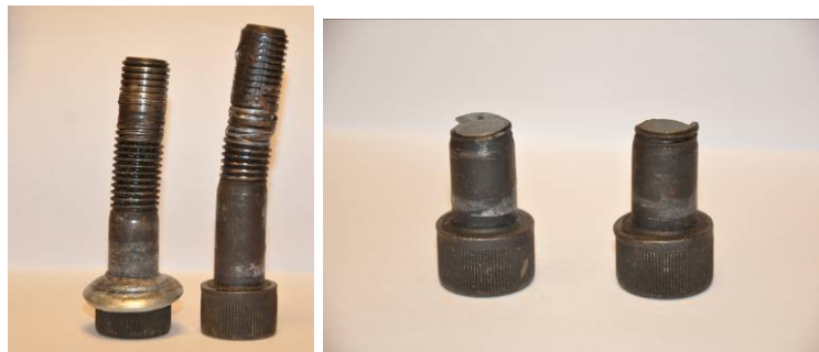
Fig. 3.24. Failure of the bolts at the link-beam connection
