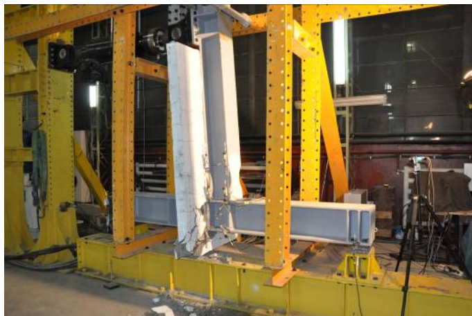
Fig. A.21. Cyclic testing of the composite joint with RBS
