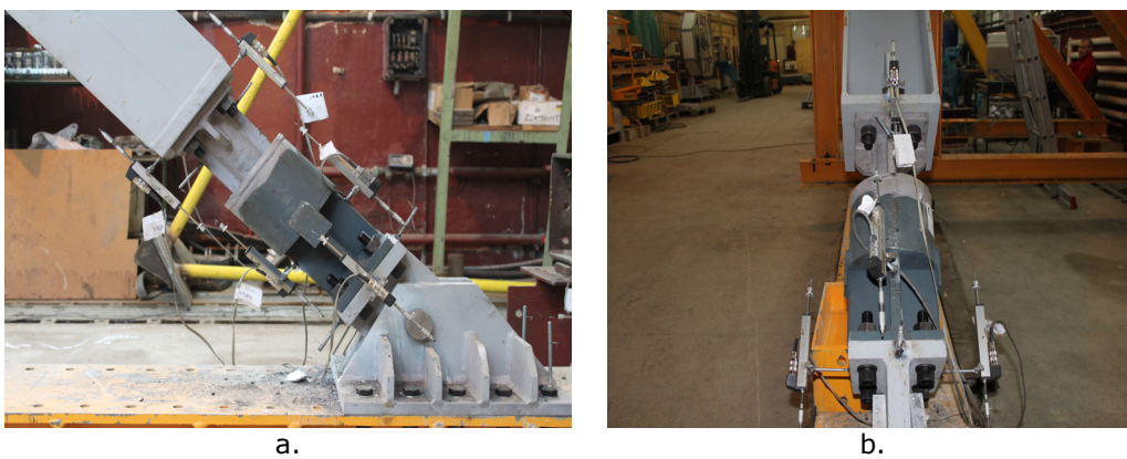
Fig. 3.21. Damper connection to brace and pinned base connection: a) lateral view; b) longitudinal view
