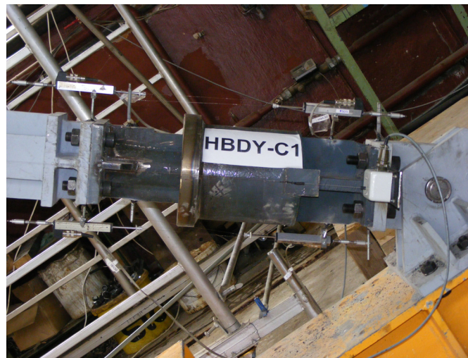
Fig. 3.12. Measurement devices positioning for the damper alone
