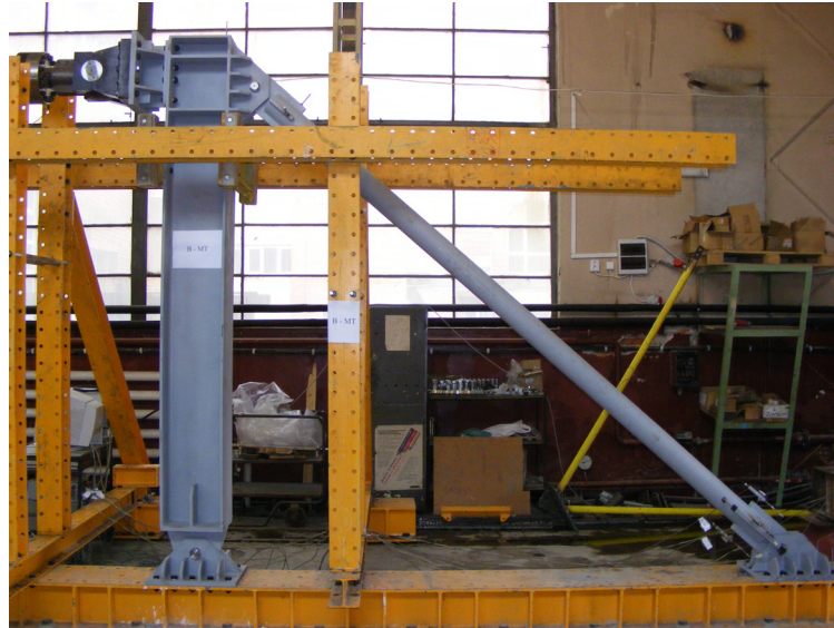
Fig. 3.23. Experimental test setup for CHS brace without damper
