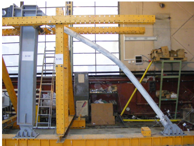
Fig. 3.26: Buckling of CHS brace under monotonic compression load
