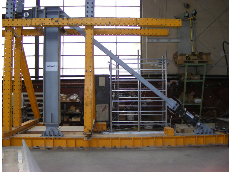
Fig. 3.41. Experimental test setup for HEA100 brace with damper specimen
