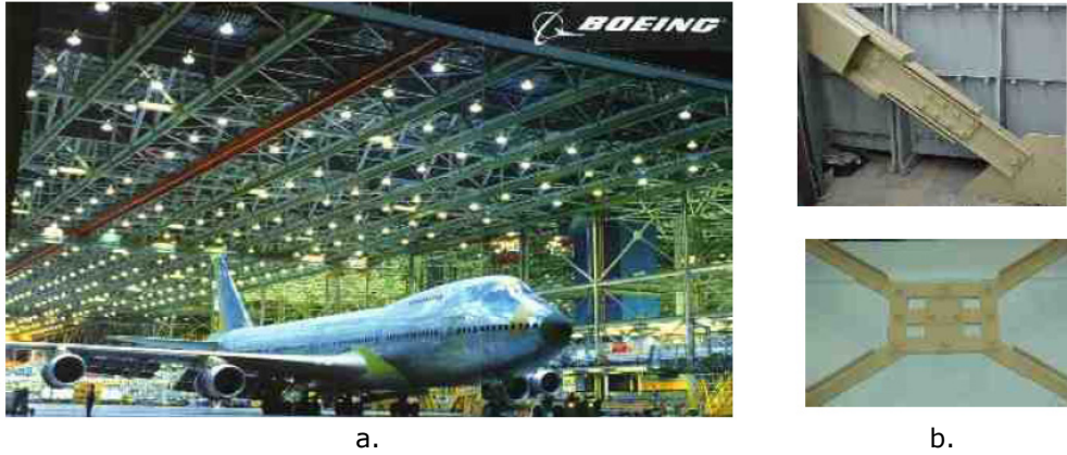
Fig. 2.33. Boeing Commercial Airplane Factory, Everett, WA, USA: a) inside view; b) Pall Friction Dampers used [26]
