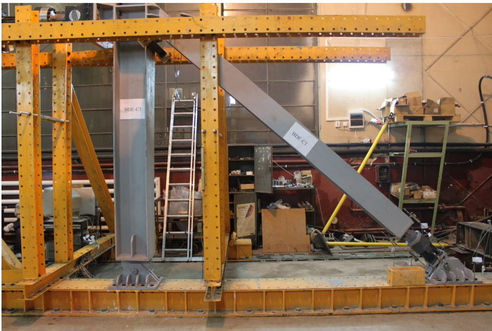
Fig. 3.19. Experimental test setup for "strong " brace with damper configuration
