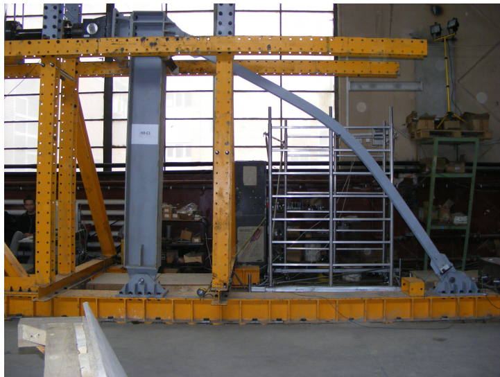
Fig. 3.39. Buckling of the HEA100 brace at cyclic tests
