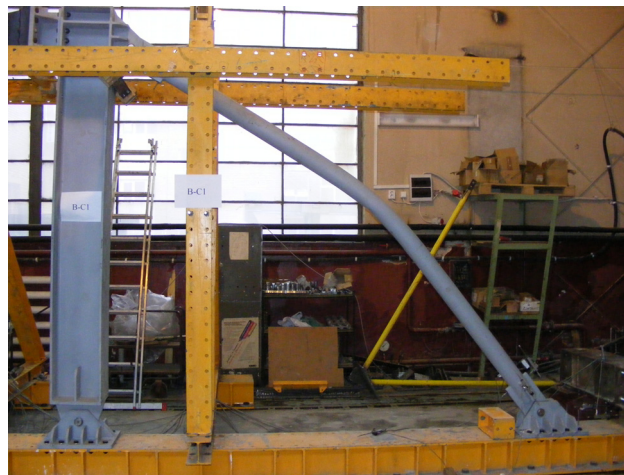
Fig. 3.29. Buckling of the CHS brace at cyclic tests
