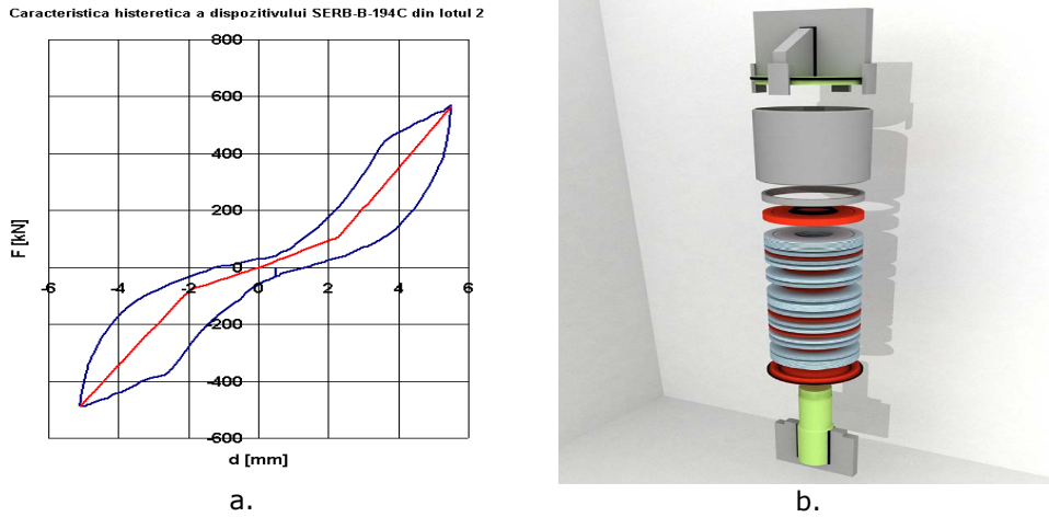
Fig. 3.1. a) Hysteretic behaviour of SERB type friction damper prototype [27]; b) SERB type friction damper components [29]
