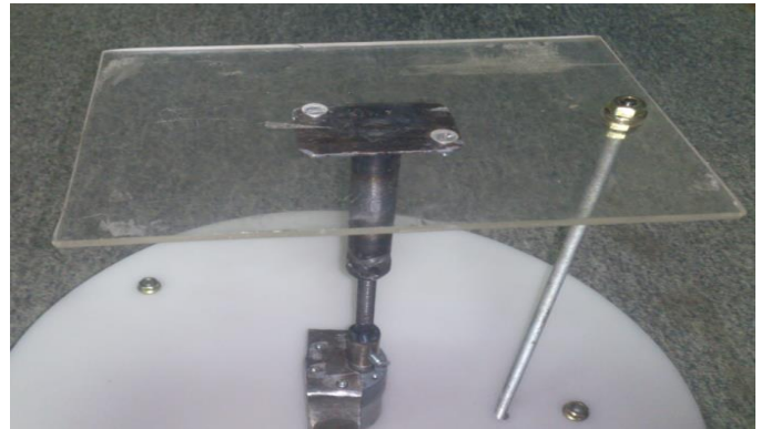
Figure 8 Cork Screw Lift Mechanism
