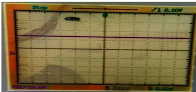
Fig. 19 Output voltage of—solar panel
