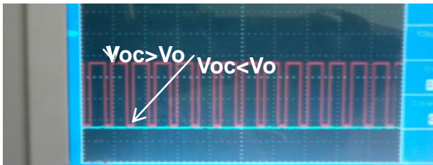
Fig 13a. Pulses generated by PIC16F877A for SMC
