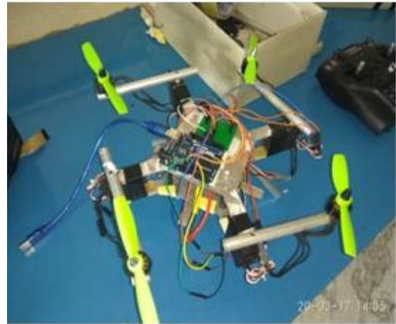
Fig 6: 90 degree retraction of arms in fold mode
