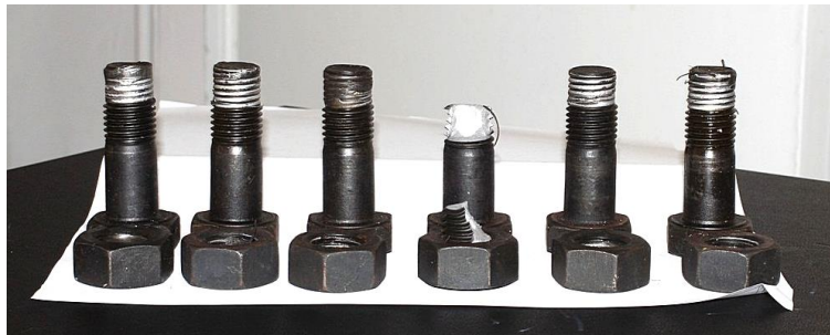
Fig. 5.10 – Failure mode for M22 bolts
