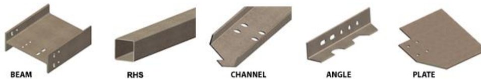
Fig. 2.1 – Regular steel cross sections
