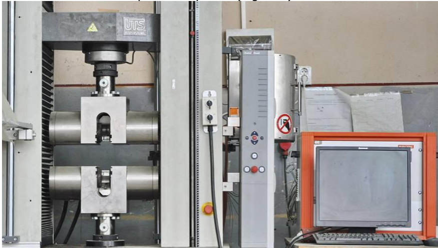
Fig. 5.2 - Universal trial device UTS/ZWICK with a capacity of 250 kN and hydraulic fixing
