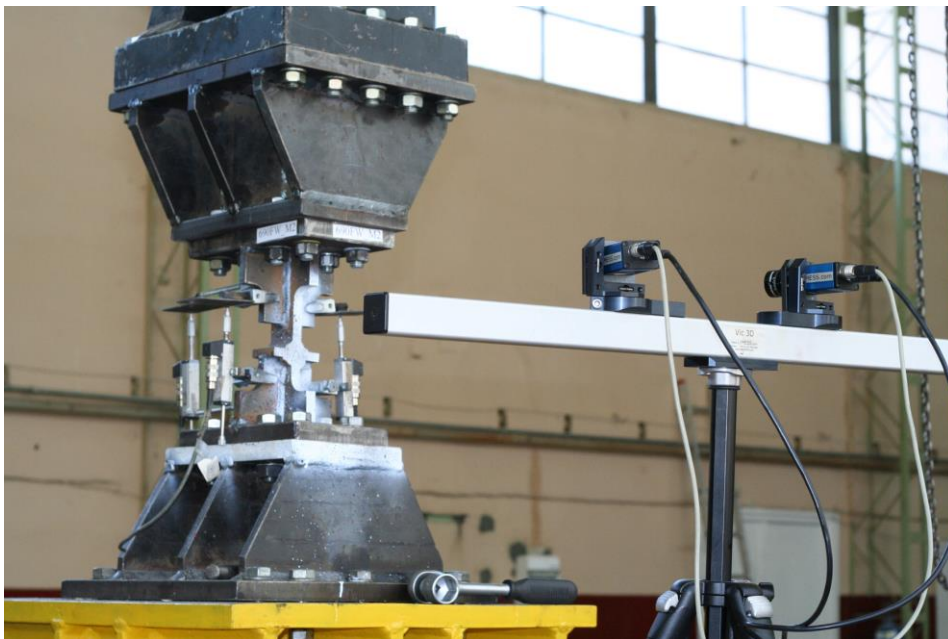
Fig. 5.14 – Welded specimen equipped with measuring devices
