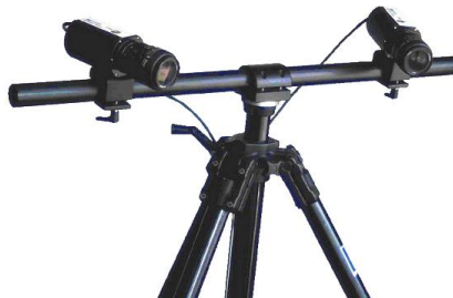
Fig. 5.4 - Digital Image Correlation system – LIMESS Vic 3D
