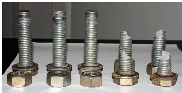
Fig. 5.9 – Failure mode for M20 bolts
