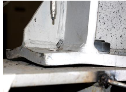
b) Experimental T-stub failure (2→1)
