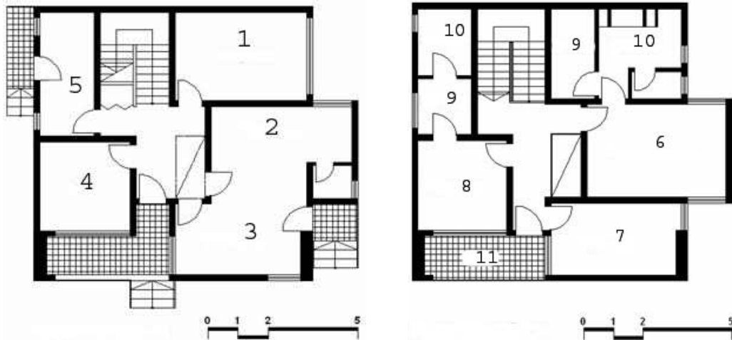
Lower floor plan: 1. dining room; 2. kitchen; 3. living room; 4. den; 5. laundry; Upper floor plan: 6. master bedroom; 7. library; 8. bedroom; 9. dressing; 10. bathroom; 11. logia
