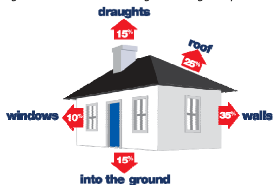
Fig. 5.61. Heat loss through building components
