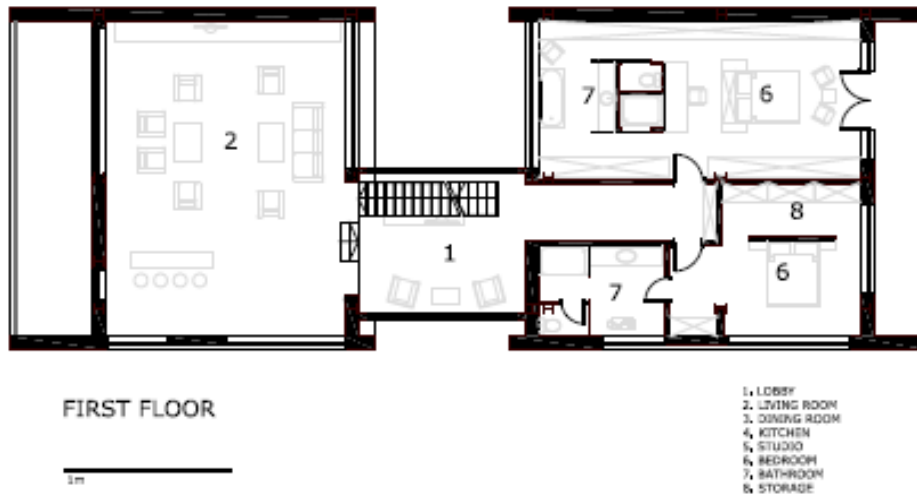
Fig. 6.38 - G House, G House - M. Mutiu, O. Gherman arch , upper floor plan
