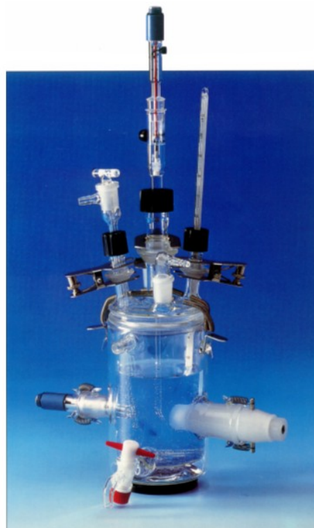
Figure 2.17 Electrochemical corrosion cell
