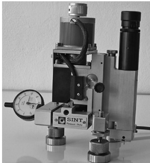
Figure 2.15 RESTAN residual stress measurement device
