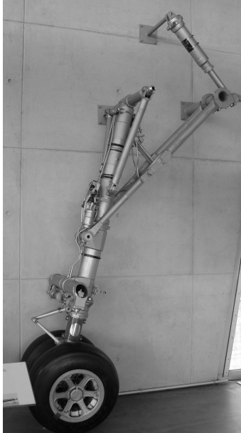
Figure 1.4 Titanium landing gear [ http://forums.pelicanparts.com ]
