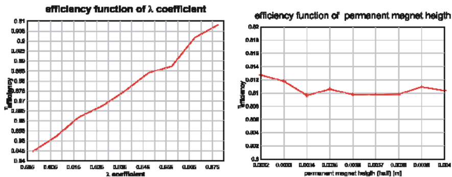
Figure 5.7: Response of the 2D equivalent FEM parameters model to a change in \lambda and permanent magnet height.
