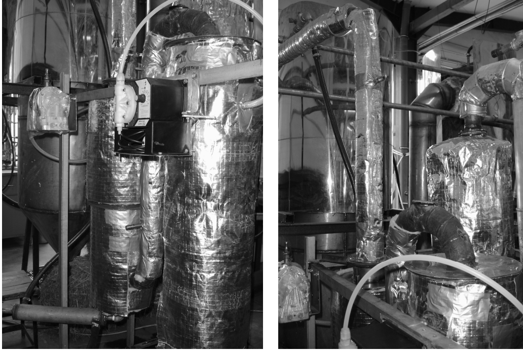
Figure E 3. \text{SO}_2/\text{CO}_2 removal system (left) view of the scrubber and absorber, and (right) top view of the columns (same as Figure 5.3)
