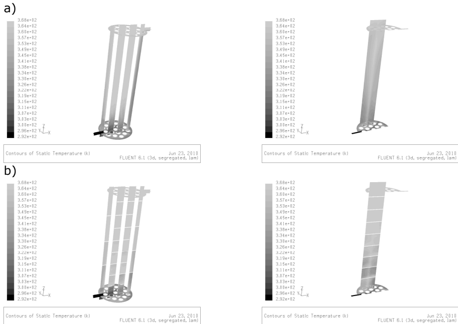
Figure E 18. Temperature contour along z -axis at different y -planes in the shell-side of heat exchanger (tube layout 30^\circ ) for water mass flow rate M \approx 26 kg/h: (a) without baffles, T_o = 361.8 K; (b) with 8 segmental baffles, T_o = 367.8 K
