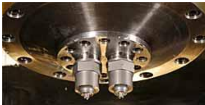
Fig. 3. 12 Twin-stir prototype head assembly
