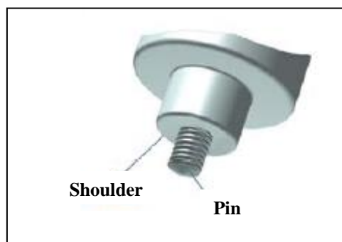
Fig. 3. 10. Schematic presentation of a FSW Tool
