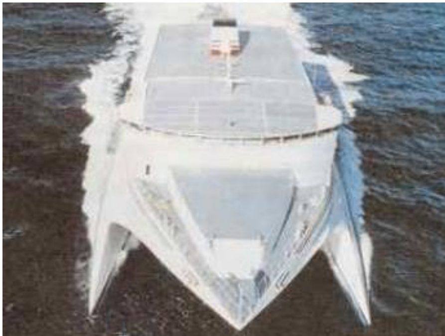
Fig. 2. 6. The use of large aluminium extrusions gives quality and cost benefits in fast multihulled catamarans.
