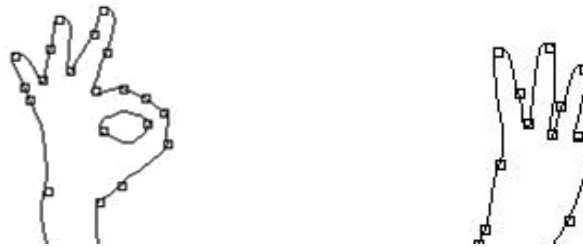
Figure 32 Examples of Harris interest points detected on hands contours
